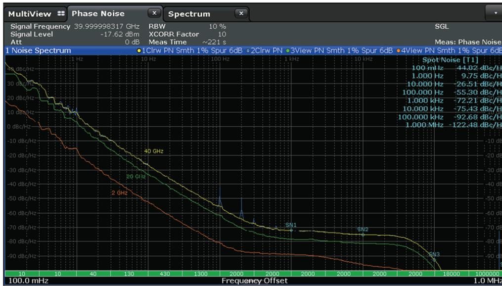
Figure 57 Some typical phase-noise values for modern synthesized signal generators (R&S).
