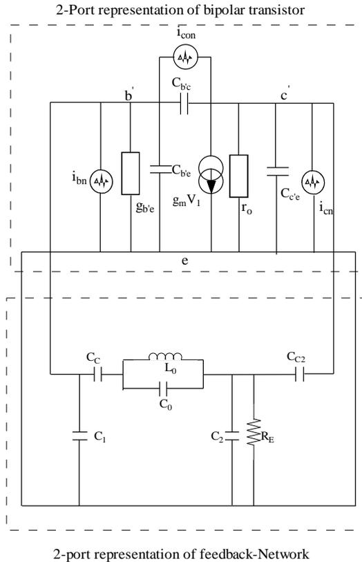
Figure 134: **Figure 21: Feedback arrangement for the Colpitts oscillator with the noise sources [5]**
