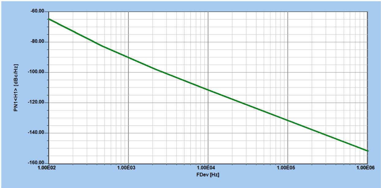
Figure 74: *Simulated Phase Noise of the 6.6GHz DRO*
