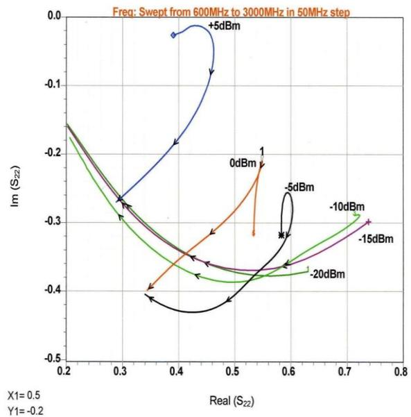
Figure 36: *Measured Large-signal S-parameters of the BFP520*
