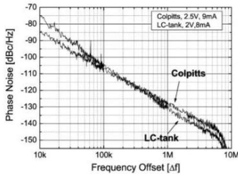
Figure 67c: Measured phase noise of a CMOS LC and Colpitts
