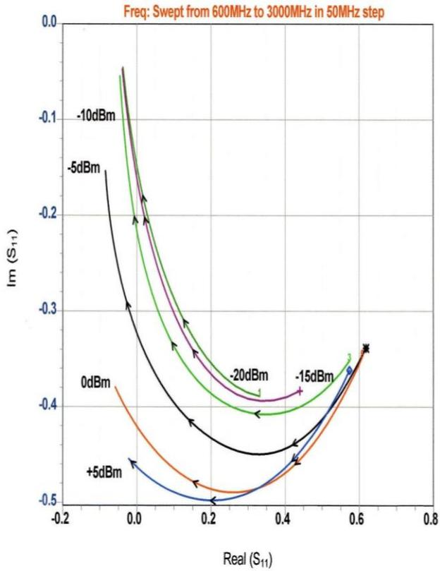
Measured large-signal  $S_{12}$  of the BFP520
