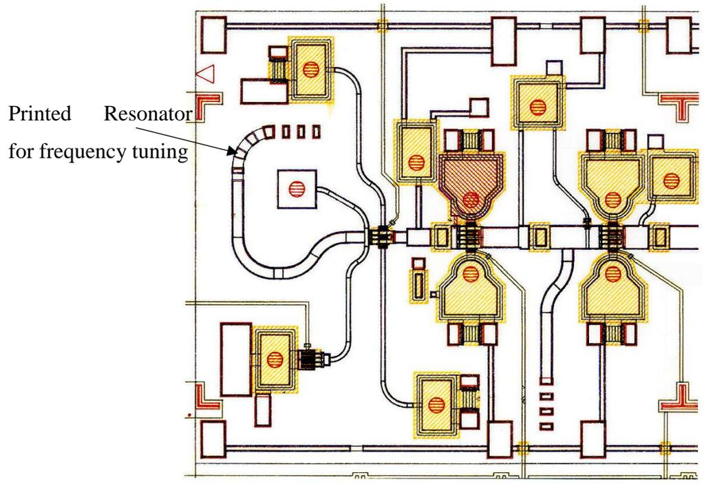
Figure 1: *Two stage FET based Microwave tunable Oscillator Built on GaAs Substrate*
