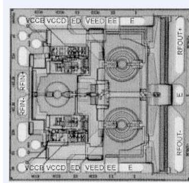
Figure 166: *Push-Pull Oscillator*
