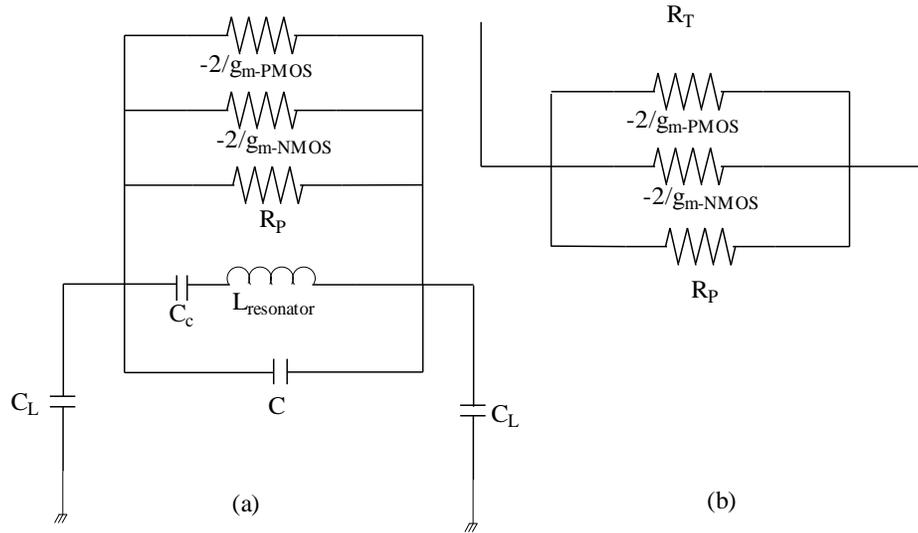
Figure 173: **Figure 8-28 a) The equivalent cross-coupled oscillator resonator circuit and b) the equivalent resistances at resonance condition.**
