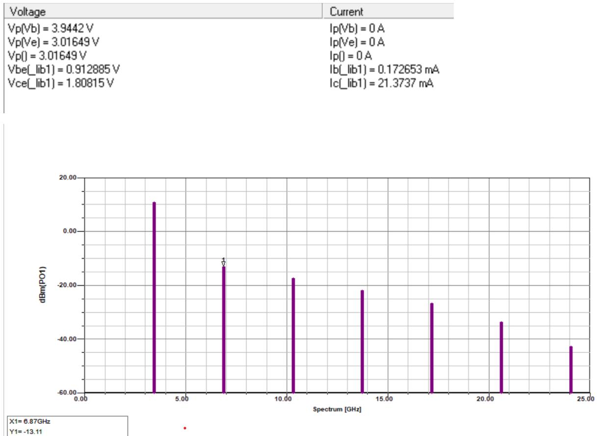
Figure 39: *Simulated Output power of the 3000 MHz oscillator using a BFP520 transistor*
