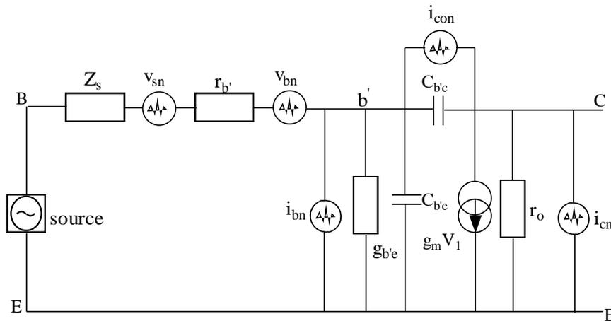
Figure 133: *Figure 20: Hybrid- $\pi$  configuration of the grounded bipolar transistor with noise sources [5]*
