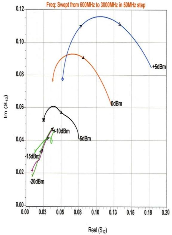
Measured large-signal  $S_{21}$  of the BFP520
