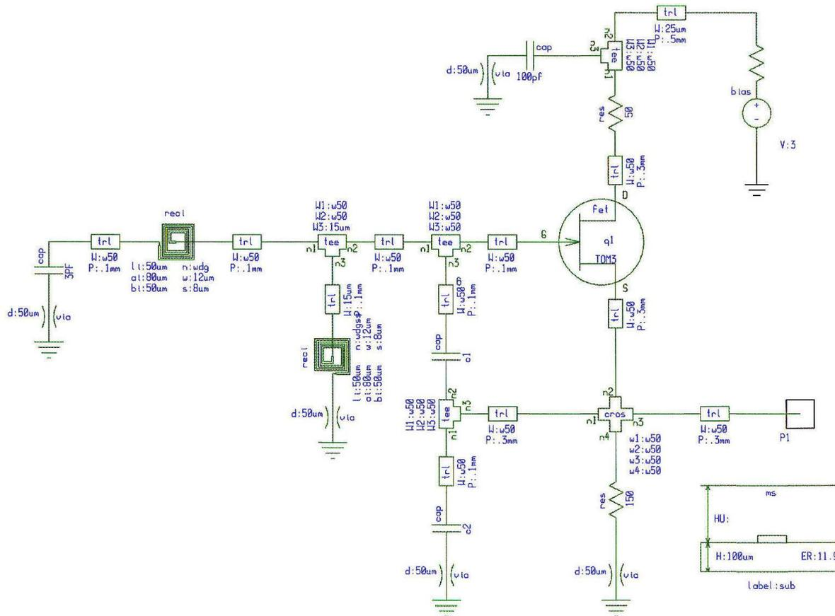
Figure 150: *Figure 9-11 Circuit schematic the 2 GHz GaAs FET oscillator built on GaAs substrate with very fine resolution of the components*
