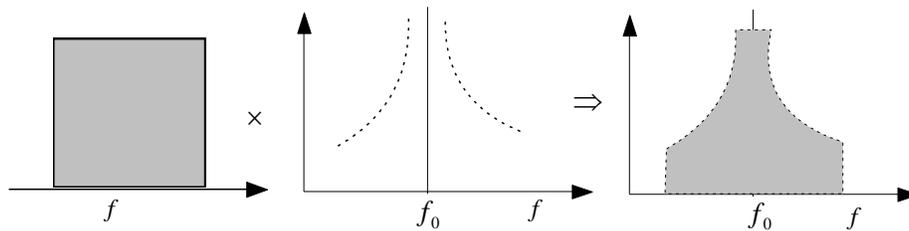
Figure 138: **Figure 25: Noise shaping in the oscillator**
