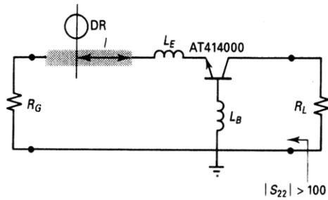
Figure 56: *Figure 4-171 Transmission line oscillator with dielectric resonator.*
