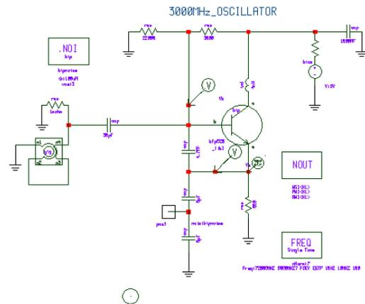
Figure 81: *Colpitts YIG oscillator*
