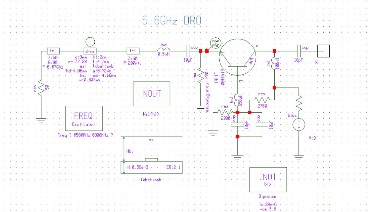
Figure 73: *Detailed Circuit schematic of a 6.6GHz DRO*
