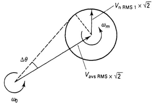
Figure 17: *Phase noise added to carrier*
