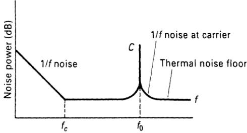
Figure 16: *Noise power versus frequency of a transistor amplifier with an input signal applied.*
