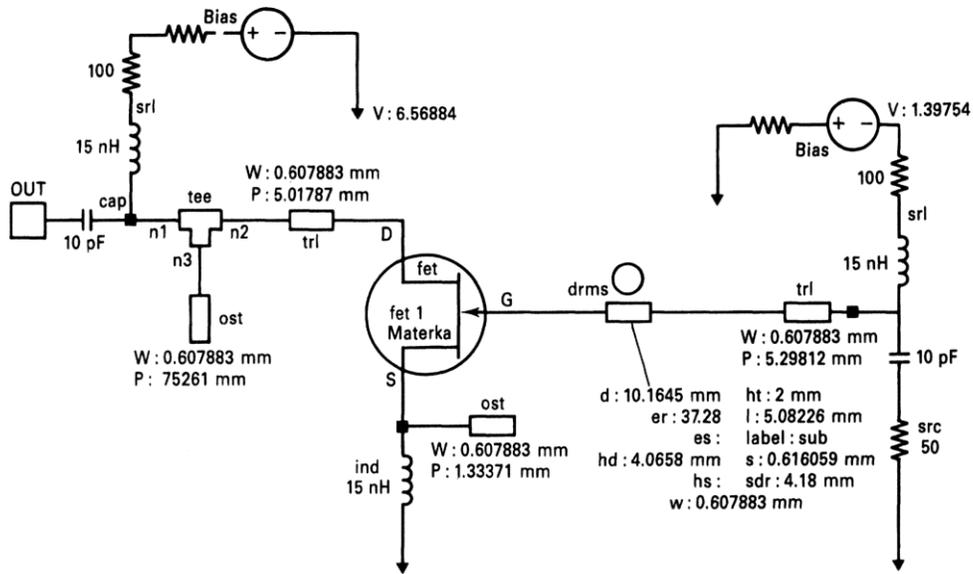
Figure 71: *Figure 4-181 Schematic of 6-GHz DRO.*
