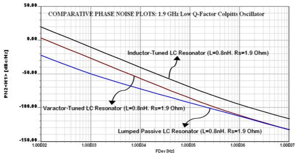
Figure 109: *This plot shows the comparative phase noise plots for the LC Colpitts oscillator using the lumped LC resonator, the varactor-tuned lumped LC resonator and the synthesized inductor-tuned resonator network for identical inductance value and loss resistance (0.8 nH with series loss resistance 1.9Ω).*
