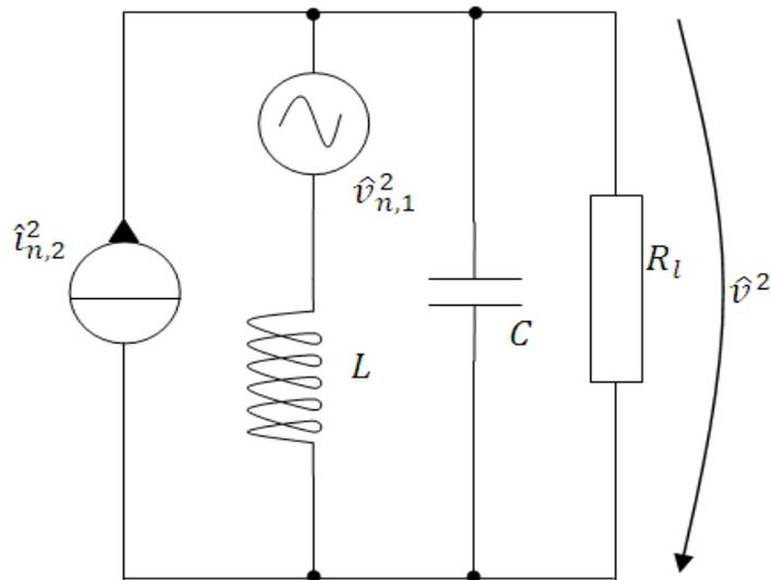
Figure 111: *Final equivalent circuit of the active inductor*
