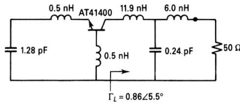
Figure 52: *Figure 4-170 Completed lumped resonator oscillator (LRO).*
