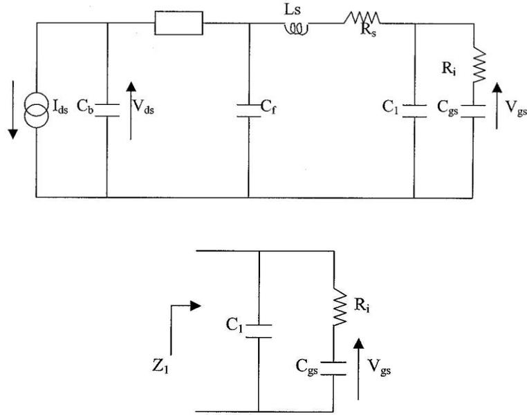
Figure 155: **Figure D-6** An equivalent circuit of the open model MESFET oscillator.
