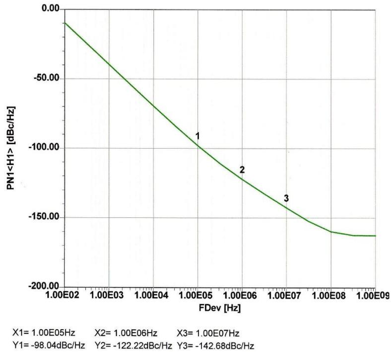
Figure 151: *Figure 9-12 Predicted phase noise of the oscillator shown in Figure 9-11. The measured values were 100 dBc/Hz at 100 kHz and 120 dBc/Hz at 1 MHz. There is a deviation of about 2 dB compared to simulation.*
