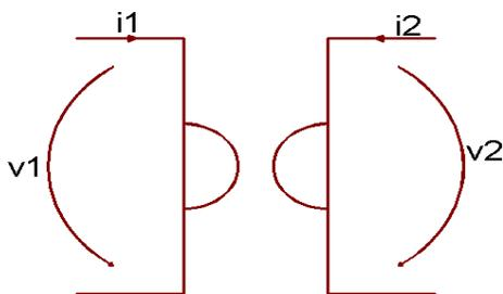
$$\begin{bmatrix} i_1 \\ i_2 \end{bmatrix} = \begin{bmatrix} 0 & g \\ -g & 0 \end{bmatrix} \begin{bmatrix} v_1 \\ v_2 \end{bmatrix} \quad \text{Where 'g' is called gyration capacitance.}$$
