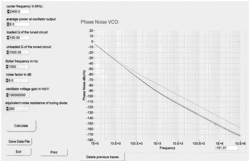
Figure 32: *Simulated phase noise following Equation (7-26).*
