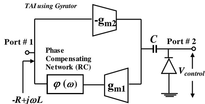
Figure 100: *Tunable Active Inductor (TAI) using Gyrator*
