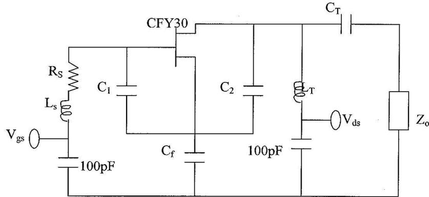
Figure 158: *Figure D-9 Schematic diagram of the oscillator operating at 950 MHz as published in [108].*
