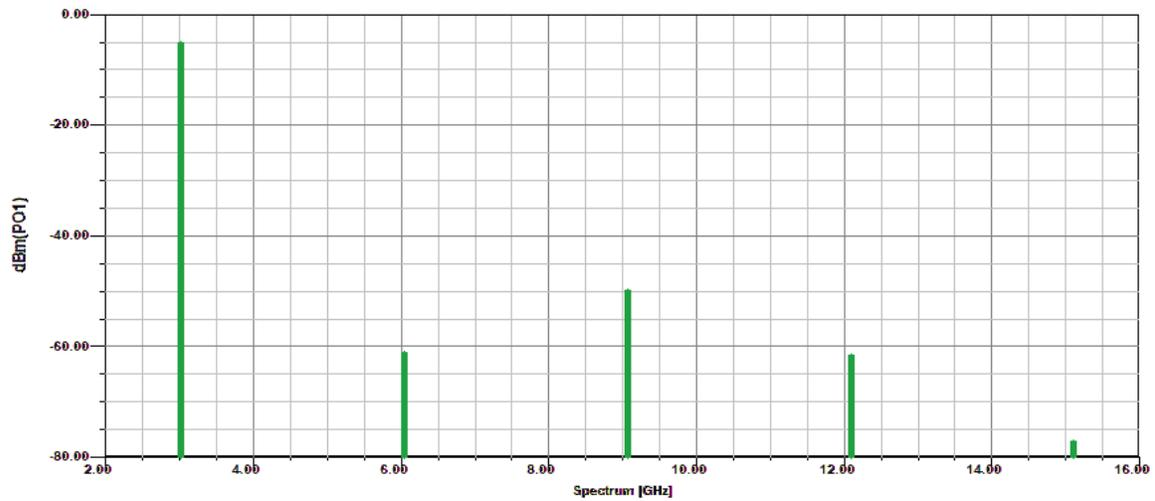
Figure 178: *Simulated output power of the CMOS oscillator*
