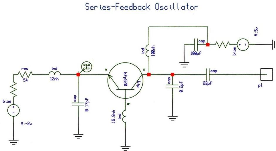
Figure 42: *Figure A-3 Shows a series feedback oscillator. For oscillation condition, the base to ground inductance and the emitter to ground capacitance is required. The 12nH inductor acts a choke. The output is tuned and terminated into 50Ω*
