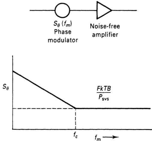
Figure 18: *Phase noise modeled by a noise-free amplifier and phase modulator*
