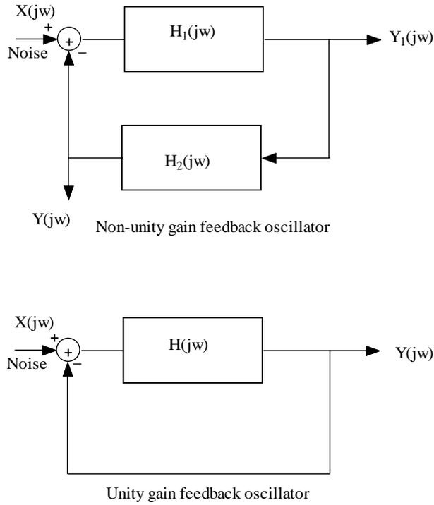
Figure 137: **Figure 24: Feedback oscillator with noise source**
