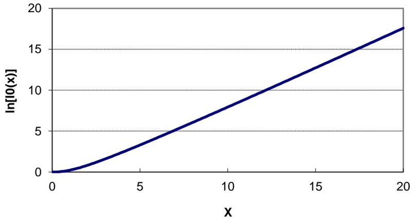
Figure 118: *Figure 6-11 Plot of  $[\ln I_0(x)]$  Vs drive level X.*
