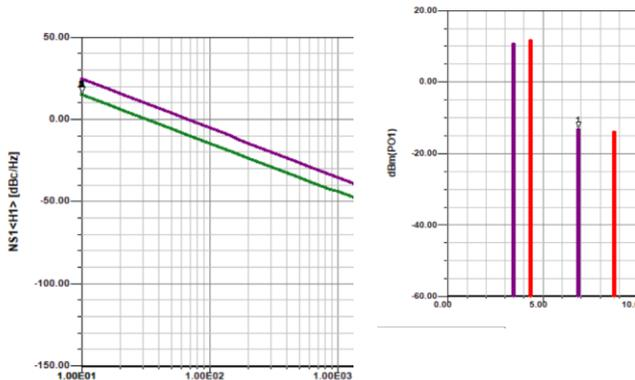
Figure 41: *Increasing the output power strongly reduces the phase noise*
