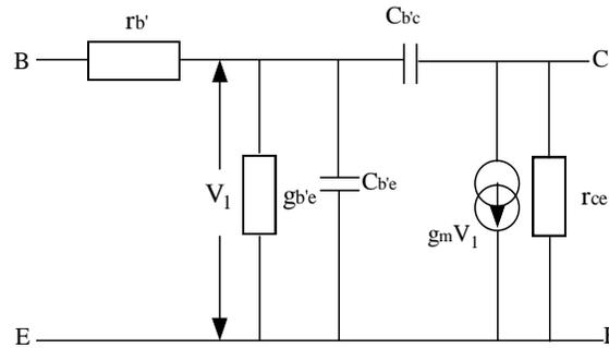
Figure 132: *Figure 19: Grounded emitter bipolar transistor [5]*
