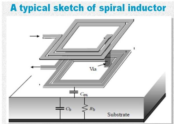
Figure 96: *A Typical Sketch of a Spiral Inductor*
