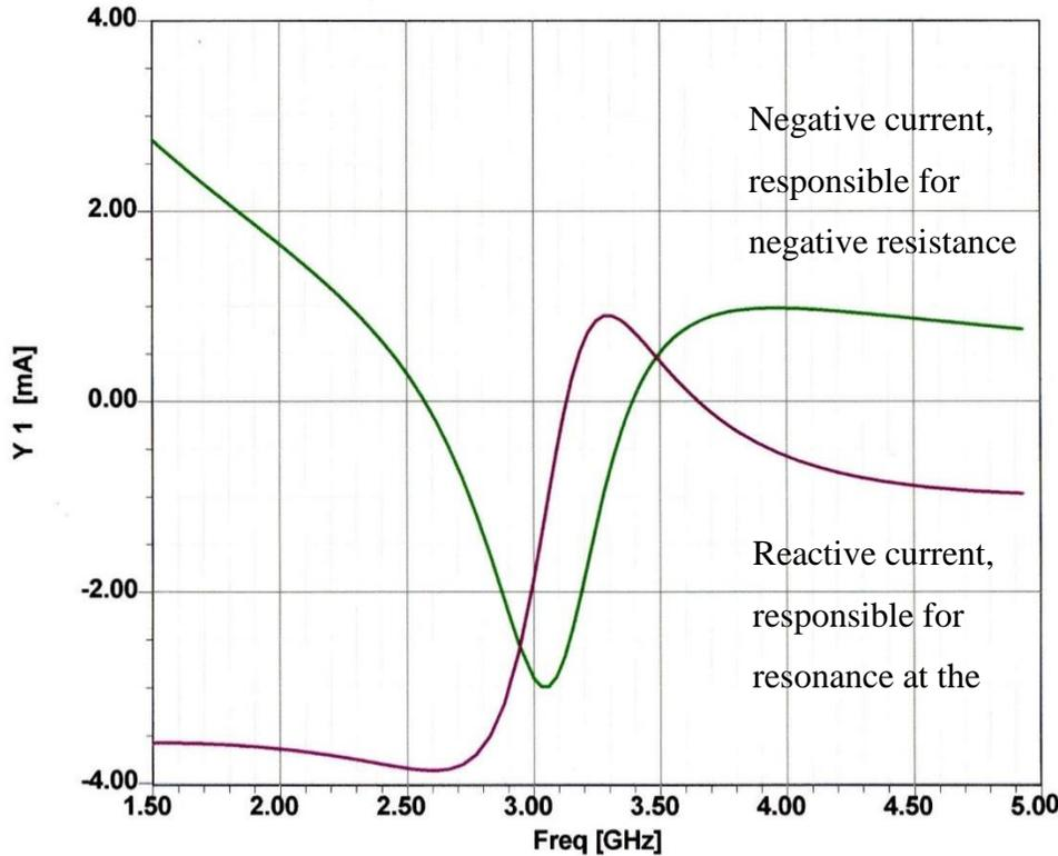
Figure 38: *Figure A-2 Shows the real and imaginary currents for oscillation. The reactive current crosses the zero line at 3120 MHz. This is close, but not exactly at the point of most negative resistance current. The reason for the shift of 120 MHz is due to the use of small-signal analysis rather than the large-signal analysis.*
