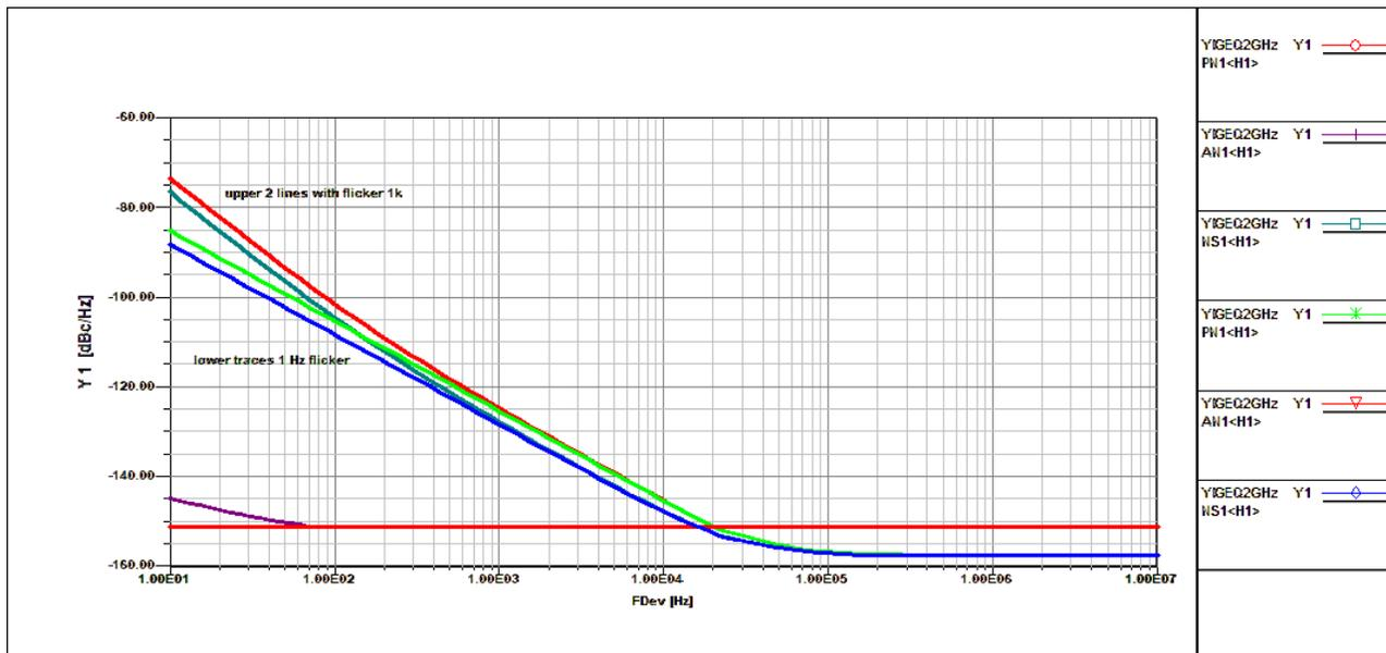
Figure 83: *Colpitts version of the Oscillator optimized - Red curve is Phase Noise dBc/Hz, dark green NS1 (Spectral Density dBc/Hz and the red one is AM Noise, also in dBc/Hz, Flicker noise set to zero*
