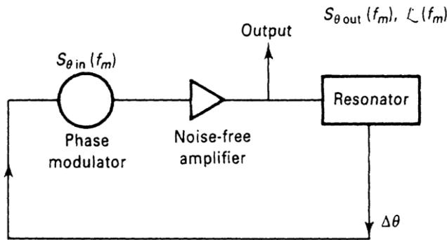
Figure 19: *Equivalent feedback models of oscillator phase noise.*
