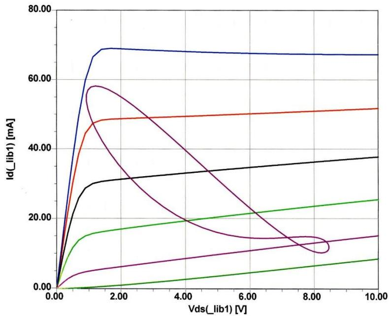
Figure 160: *Figure D-11 Load line of the oscillator shown in Figure D-10. Because the load is a tuned circuit, the “load line” is a curve and not a straight line.*
