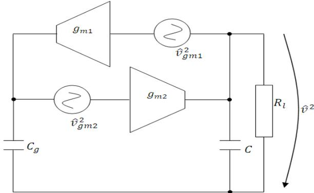
A simplified circuit of active inductor resonator with noise
