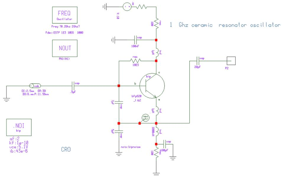
Figure 91: *Figure 4-190 Schematic of the ceramic resonator-based oscillator.*
