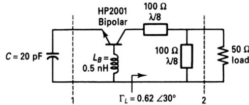
Figure 45: *Figure 4-167 Oscillator example at 2 GHz.*
