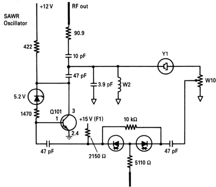
Figure 64: *Figure 4-177 Schematic of a SAW oscillator.*
