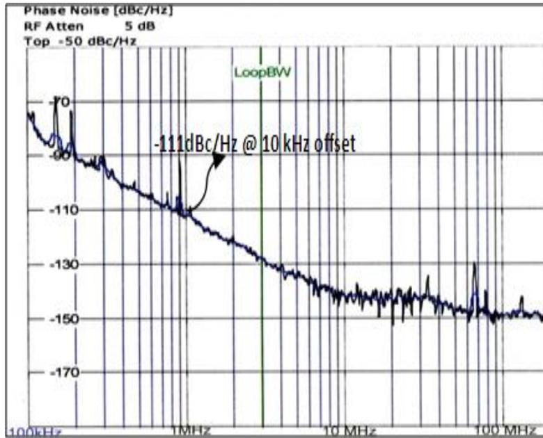
Figure 116: *Measured Phase Noise of the .....*
