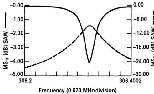
Figure 63: *Figure 4-176 Frequency response of a SAW oscillator.*
