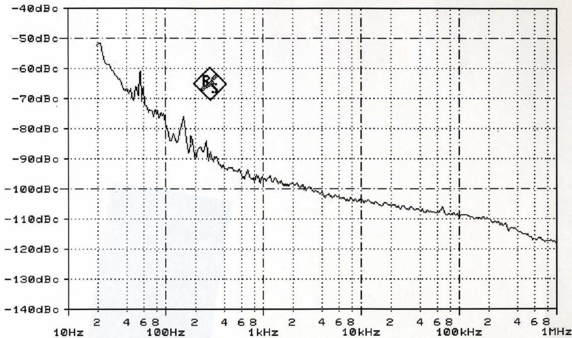
Figure 27: *Typical phase noise of a PLL 50 GHz PLL synthesizer*
