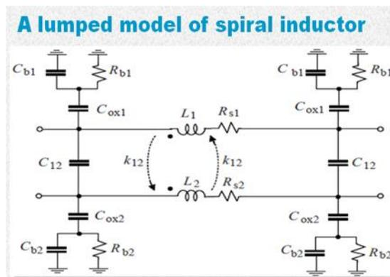
Figure 97: *A Lumped Model of Spiral Inductor*
