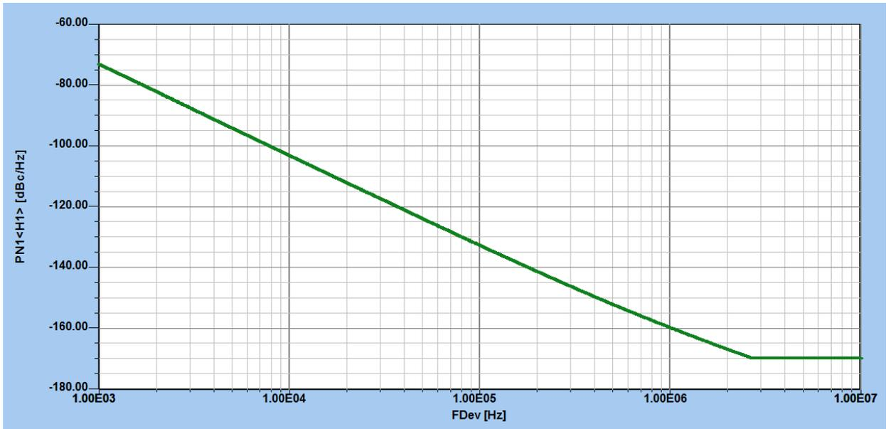
Figure 53: *Simulated Phase noise of the 4-GHz lumped resonator oscillator*
