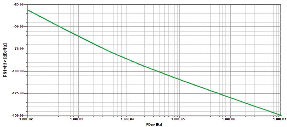
Figure 179: *Simulated phase noise of the CMOS oscillator*
