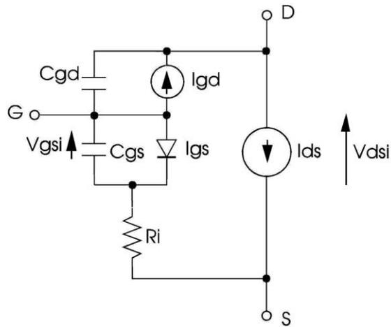
Figure 11: *Figure 3-12 Topology of the intrinsic model.*
