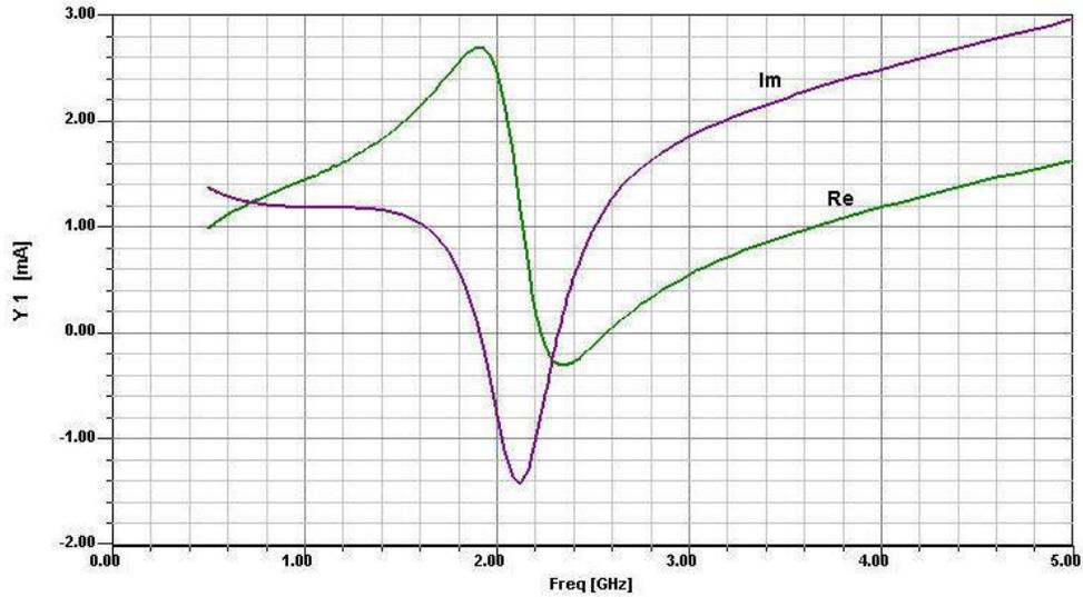
Figure 169: *Figure 8-24 The real and imaginary currents which causes the negative resistance for oscillation.*
