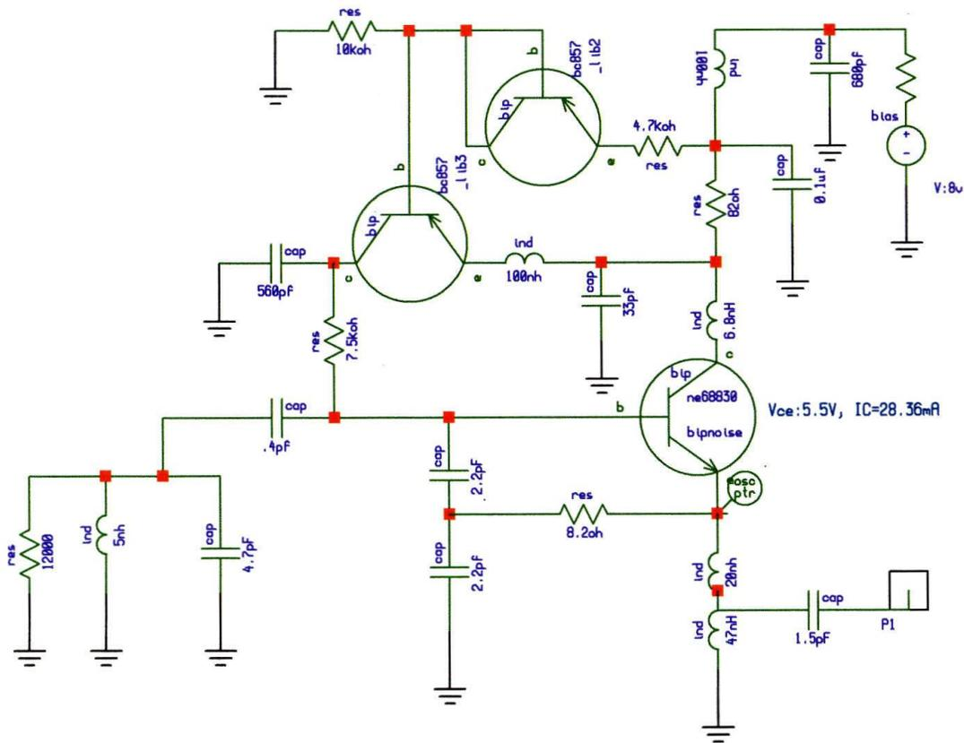
Figure 144: *Figure C-1 Schematic of the 1000 MHz oscillator.*
