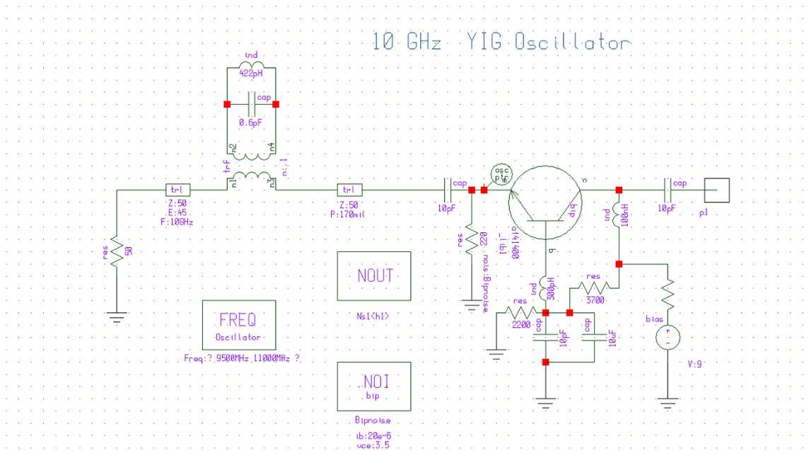
Figure 80: *10GHz YIG based oscillator with base-inductor feedback*
