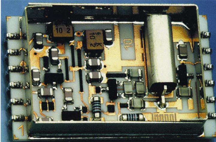
Figure 143: *Figure C-1 shows the parallel-tuned Colpitts oscillator circuit, which has to be designed with the following specifications. The unit was also built and measured. It uses a ceramic resonator and its equivalent circuit is shown.*
