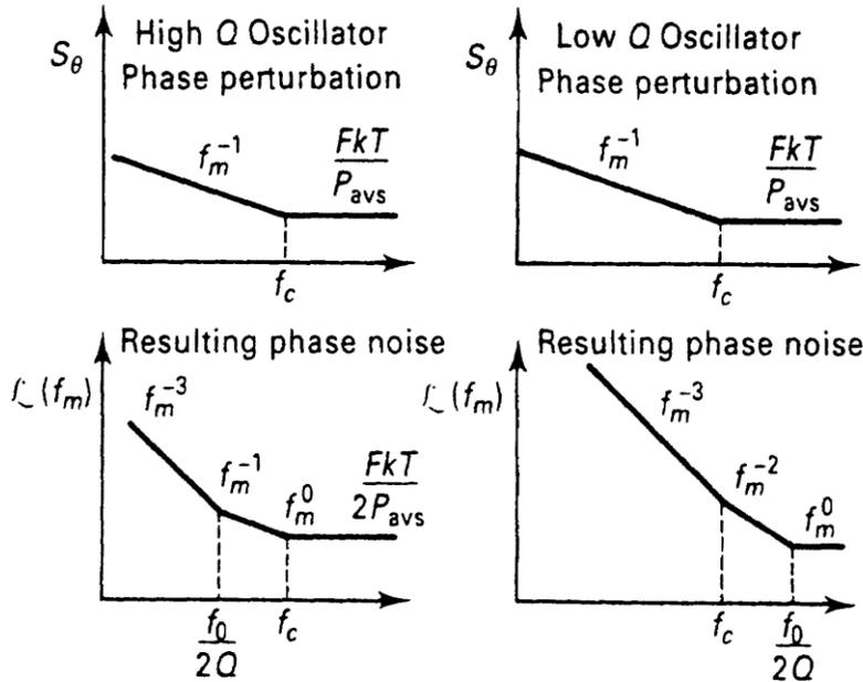
Figure 20: *Equivalent feedback models of oscillator phase noise.*
