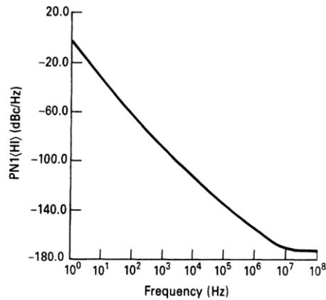
Figure 72: *Figure 4-182 Predicted phase noise of the 6-GHz DRO pictured in Figure 4-181.*
