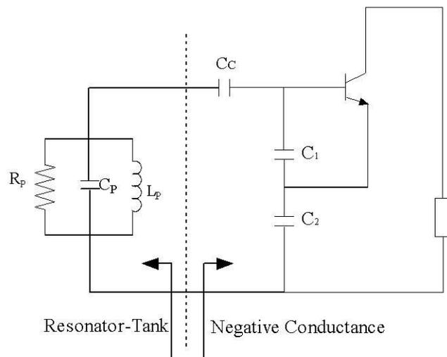
Figure 129: *Figure 8-2 Colpitts Oscillator configuration for the intrinsic case, no parasitics assumed, and an ideal transistor considered.*
