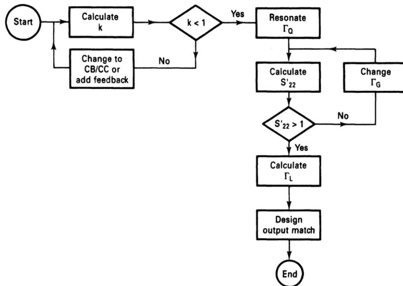
Figure 46: *Figure 4-168 Oscillator design flowchart.*
