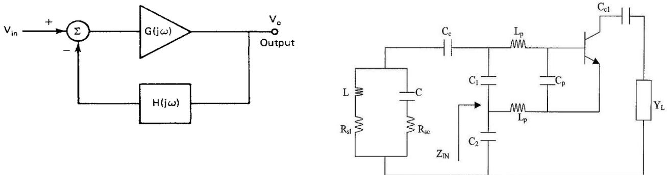
Figure 30: *Oscillator as a feedback model and as a one port producing a loss compensation with the electronically generated negative impedance.*
