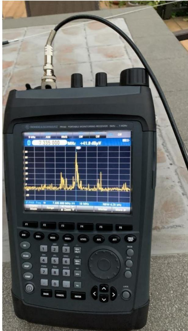
Then the Manpack, using the build in tuner was matched with a mobile antenna. This resulted in the same 1 dB $\mu$ V noise level. A short wave receiver typically has a noise figure of 10 dB without a pre-amp or 10 dB S/N at 0.3  $\mu$ V, or -10 dB $\mu$ V. At this 1 dB $\mu$ V level a 10 dB $\mu$ V signal is needed. And yes, 28 MHz or even 50 MHz is much quieter,
