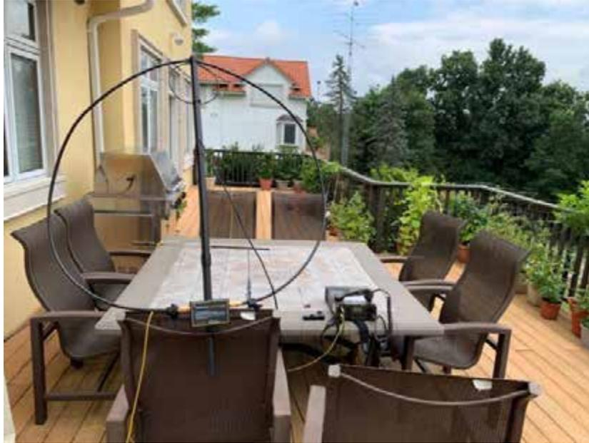
The small HF loop, an AlexLOOP, pictured above has efficiency shown in the figure below.
