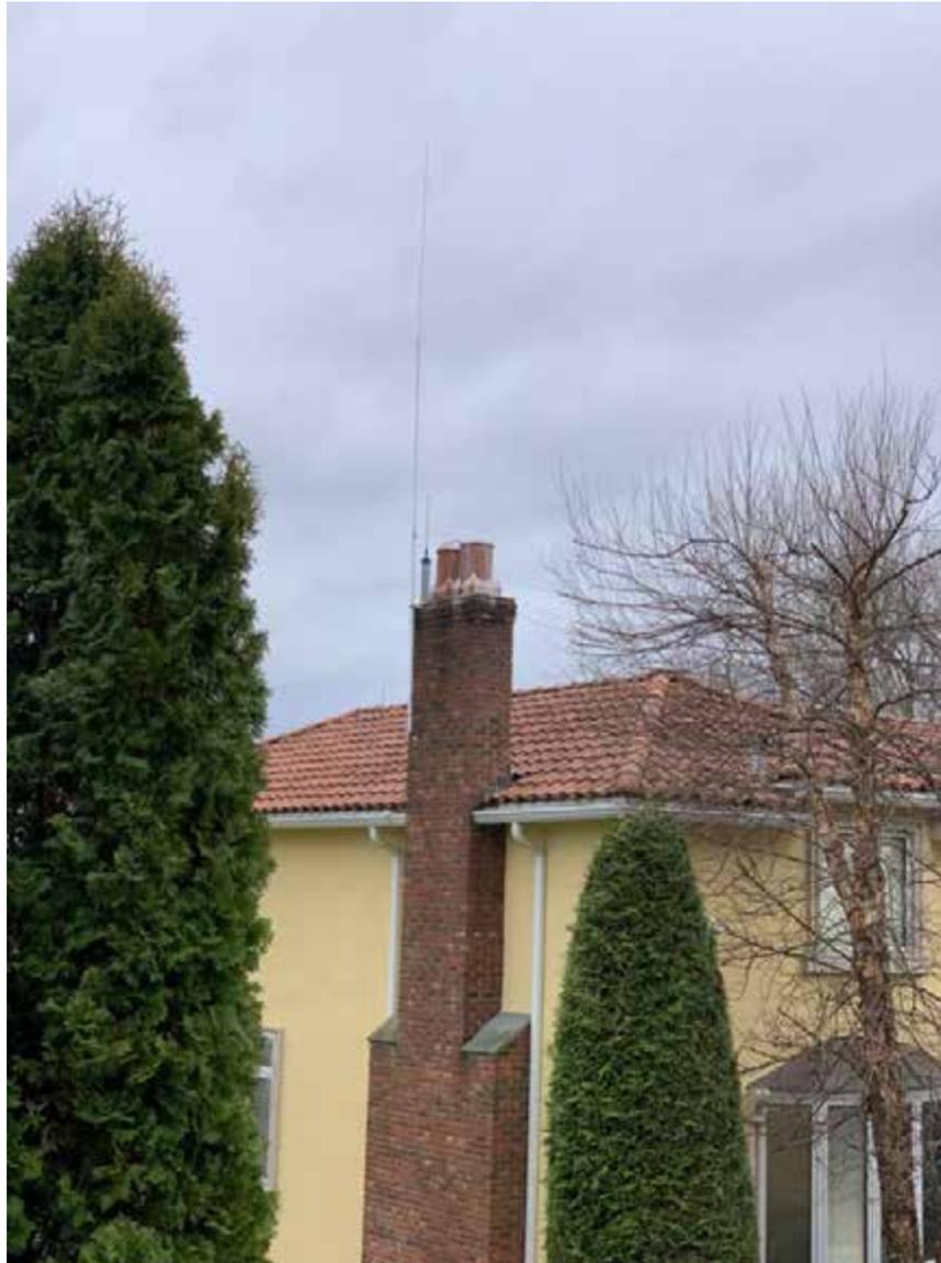
Vertical rod or whip antennas have their place, as seen above, this vertical is driven by an antenna tuner, it works very well from 7 MHz to 50 MHz. For amateur bands 1.8 to 4 MHz it's a bit short, but given the environmental noise it works sufficiently well in receive. In transmit the efficiency is about 2.5 %. This antenna will also be used to compare with the small HF loop antenna operating above 7 MHz.
