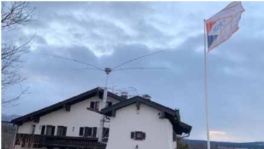
That is, each side has two dipole which puts the antenna in the category of two thick dipoles or fan dipoles. In the background for DX operation is the StepperIR antenna and the vertical antenna is “hidden” in the flagpole.
