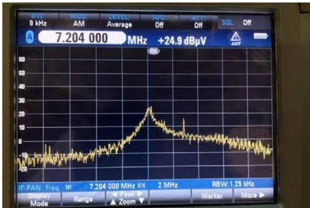
When the loop antenna is used, the wide band noise is multiplied with its narrow band width and we see the noise peak, resonant condition
