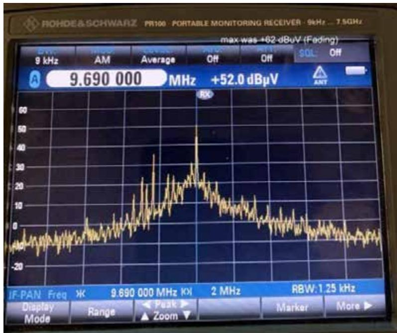
Tuning the loop antenna to the 30 m broadcast range the wanted signal at 52 dBuV shows the peak while the high Q suppresses the adjacent signals.
