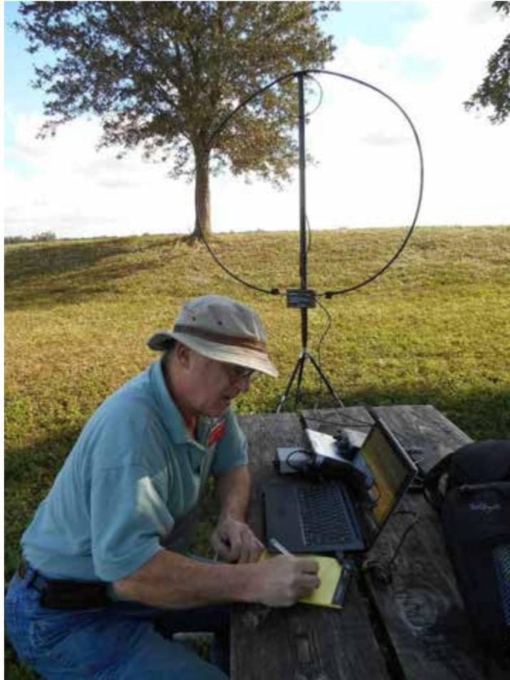
Kai Siwiak, KE4PT, shown using a small HF loop in a portable station at a public park.
