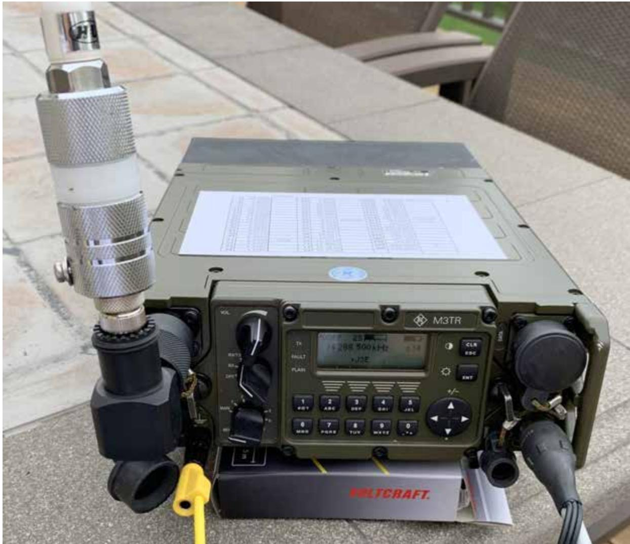
The yellow wire is a “counterpoise” of 5 m length. The displays shows 25 dB $\mu$ V; C14 refers to the channel 14, which happens to be in the 20 m band , tunable in 1 Hz steps, and +J3E refers to upper side band .
