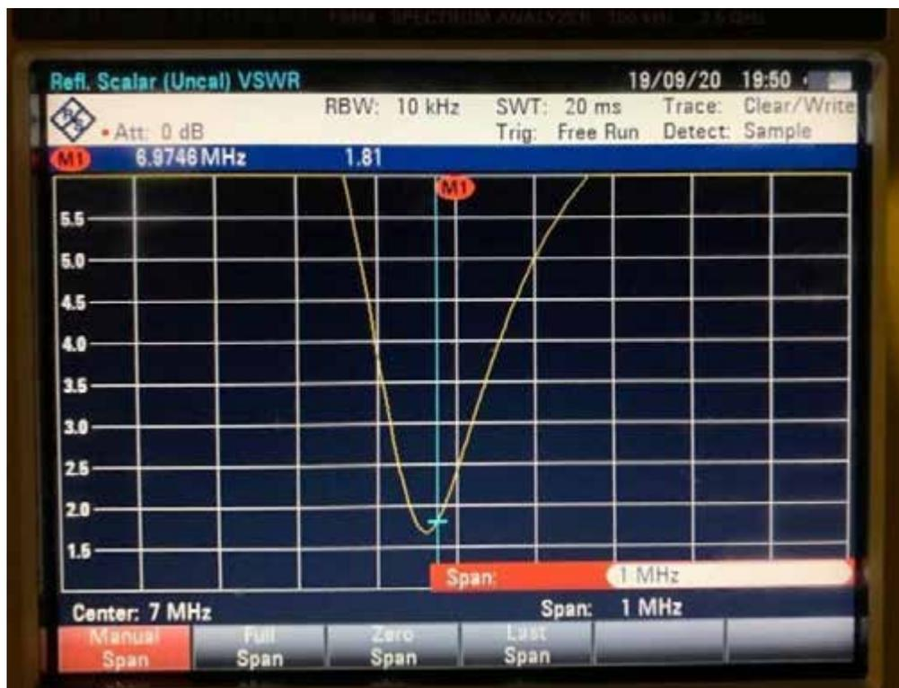
This measurement is actually tricky as the R&S network analyzer model FSH4 needs to have a proper counterpoise or set of radials. A somewhat simpler test is to check if the resonant frequency varies if the analyzer is touched. In this case two resonant cables were used like a set of radials.
