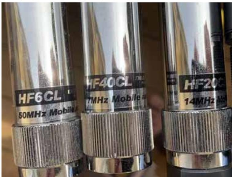
Relative to an SWR of 2.6 dB, 3dB bandwidth the loaded Q is  $6.975 \text{ MHz}/110 \text{ kHz} = 63$ .
