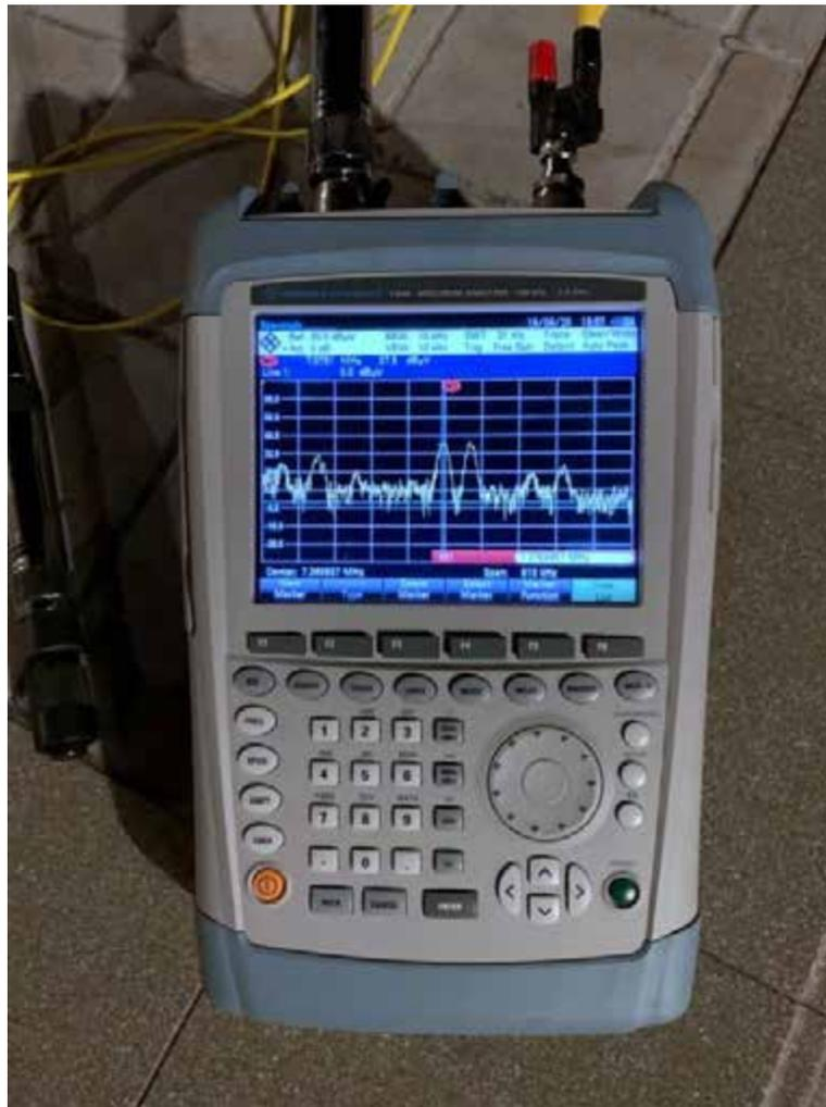
The peak signal was a French language station at 7.375 MHz peaking 48.5 dB $\mu$ V while the same station at the 8 m marine whip antenna was 75 dB $\mu$ V, see below
